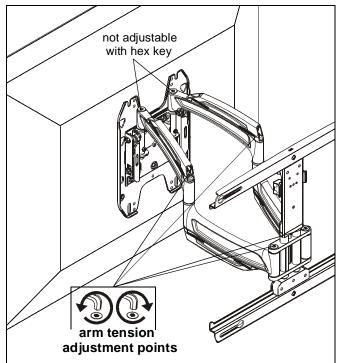
2. Use 9/16" wrench to adjust arm tension directly behind faceplate. (See Figure 35)
