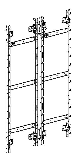
LOOSELY INSTALL THE 1/4-20 BUTTON HEAD CAP SCREW AND WASHER. THEN SET THE NEXT SECTION INTO PLACE
