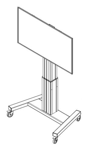
Motorized mobile trolley for large size and touch screens up to 100" and 150Kg.
